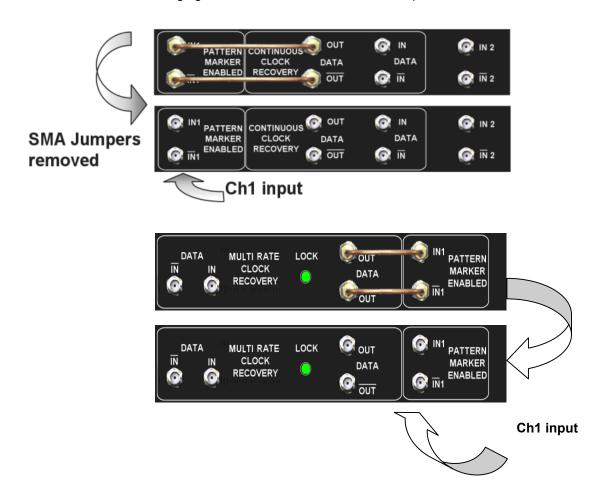
The final instructions will prompt to reconnect the jumpers, follow the on-screen directions for specific connections.
