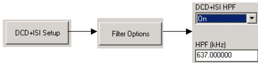
**Figure 17 - DCD+ISI High Pass Filter Settings**
