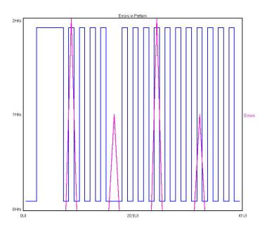
Figure 1(a) shows a plot of the pattern and the number of errors for each bit in the pattern. In this example there are six bit errors at four different bits in the pattern.
